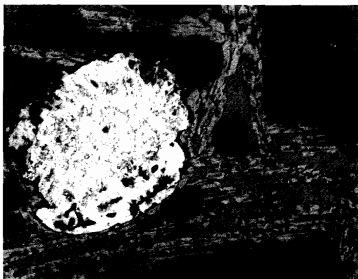
Figure 19. Structure of high carbon piece of steel entrapped in slag (no. 67): pearlite matrix. Etched in 4 per cent nital. (x100)
