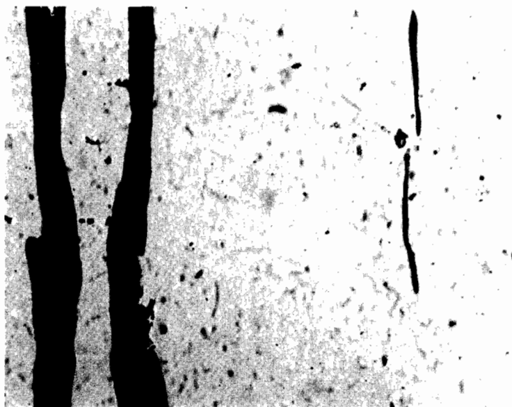
Figure 13. Structure of one-phase slag inclusions resolved at high magnification. Uniformly black single-phase glassy stringers. As polished (not etched). (x500)
