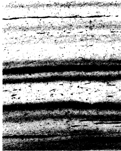
Figure 16. Banded structure in wrought iron. Phosphorus-rich bands (light) and phosphorus-poor bands (dark) of ferrite, slag stringers (black). Etched in Oberhoffer reagent. (x50)
