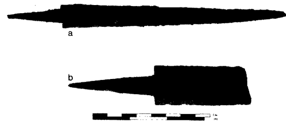
Figure 15. Files: a) warding file with illegible mark, IH51J2-1; b) 1/2-round, double-cut file, broken on shaft, marked "MV&amp;Co," IH51L5-1. (Photo by R. Chan)
