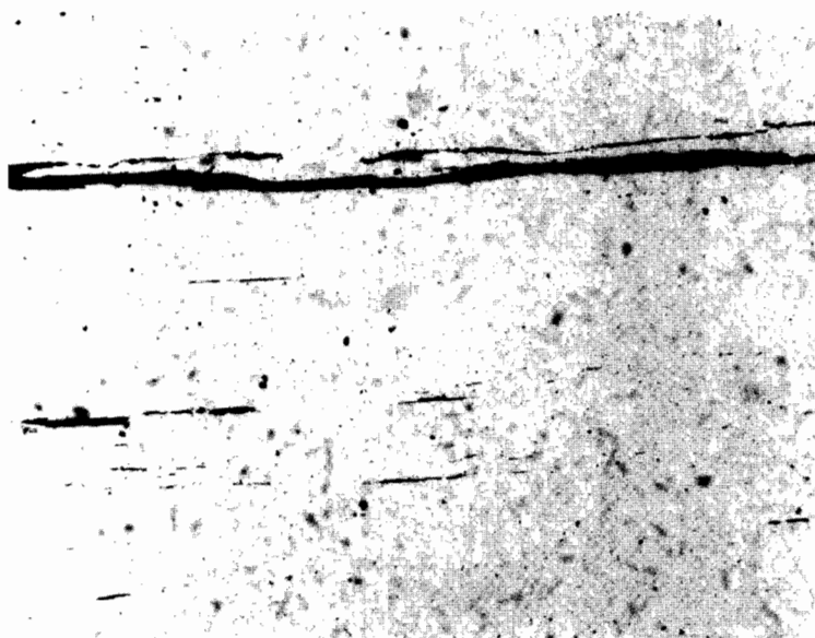
Figure 11. Very long and thin slag stringers (black) of one-phase structure. As polished (not etched). (x100)
