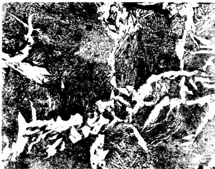
Figure 22. Figure 21 at higher magnification. Coarse lamellar pearlite (dark-light) resolved, and grain boundary ferrite (light). Etched in 4 per cent nital. (x500)
