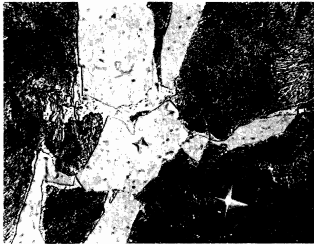
Figure 26. Figure 25 at higher magnification. Massive cementite crystals (946 HV 100 ) in matrix of lamellar pearlite (254 HV 100 ). Etched in 4 per cent nital. (x500)
