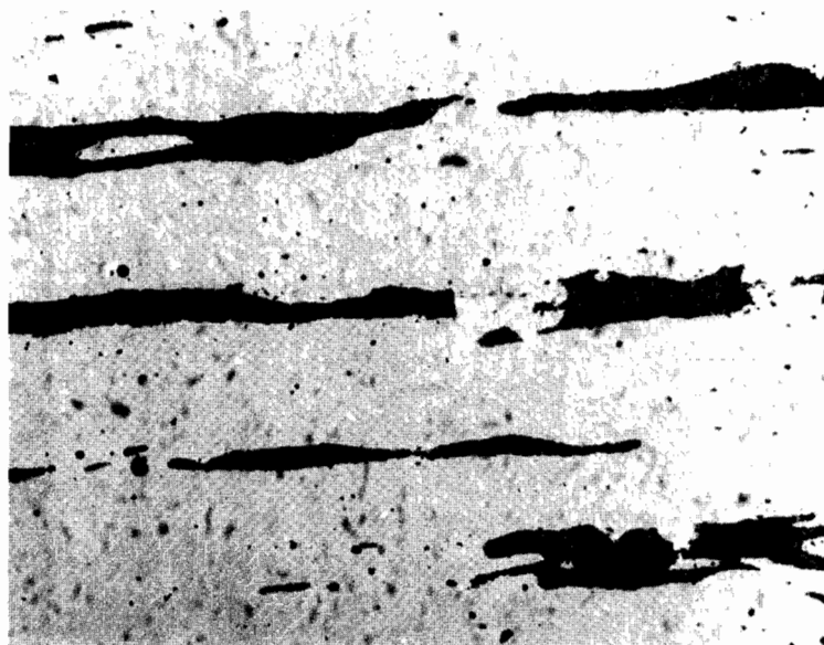
Figure 10. Large slag stringers (grey) of two-phase structure. As polished (not etched). (x100)
