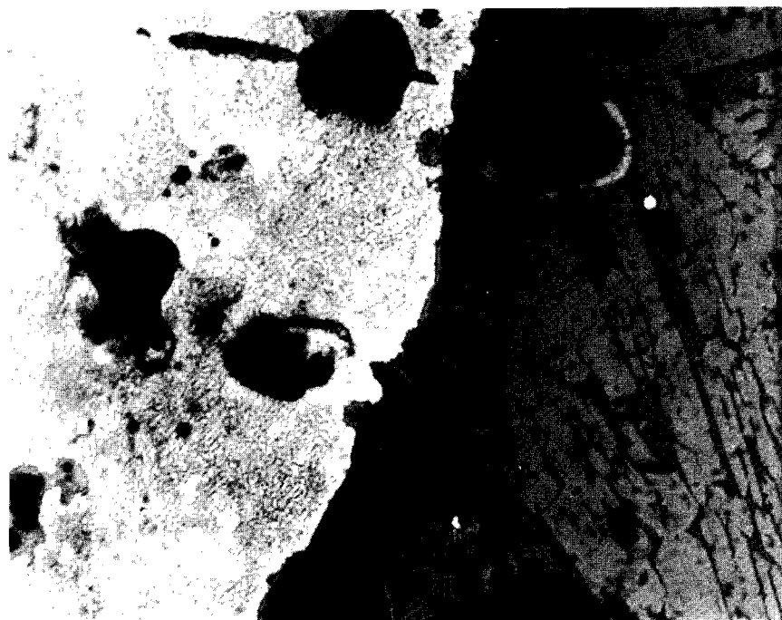
Figure 20. Structure of high carbon piece of steel ( left ) entrapped in slag (no. 62): unresolved pearlite. Etched in 4 per cent nital. (x150)
