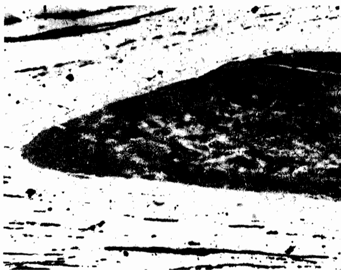
Figure 27. Forge-welded steel bit (dark) to wrought-iron blade (light) in axe head 1H51G3-9. Etched in 4 per cent nital. (x25)
