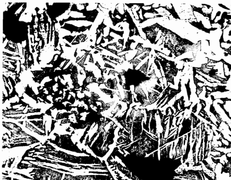
Figure 18. Widmanstaetten structure of medium carbon piece of steel entrapped in slag (no. 7): ferrite (light) at grain boundaries and within grains, in matrix of pearlite (dark). Etched in 4 per cent nital. (x100)
