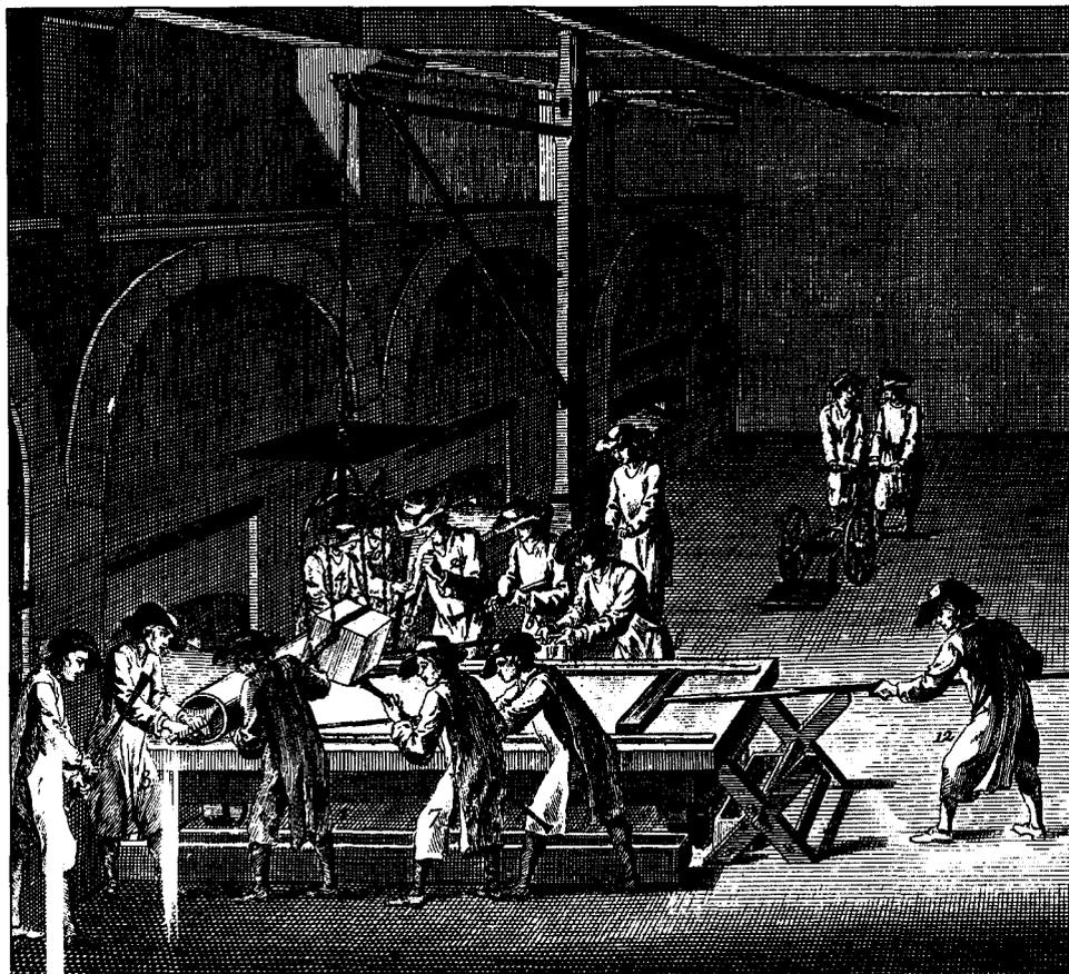
26 Plate glass. The molten glass is being poured onto the casting table and rolled. Denis Diderot, *Pictorial Encyclopedia of Trades and Industry*, Plate 273.
