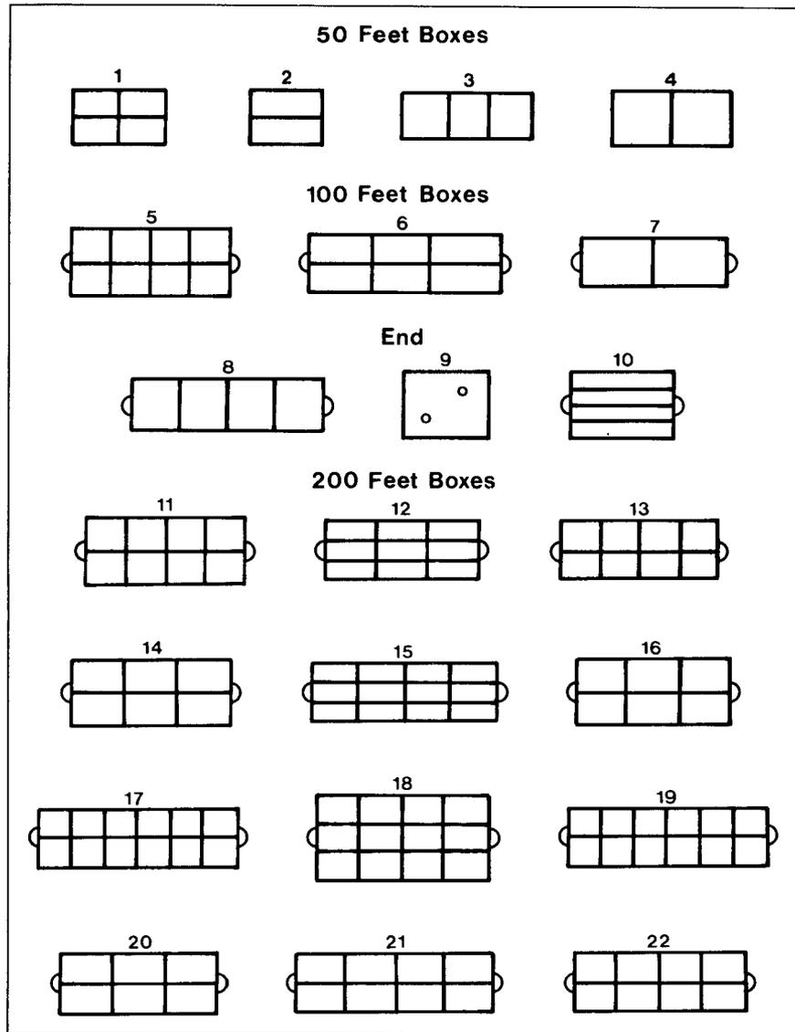
**29** Boxes to contain 50, 100 and 200 feet of glass, showing where the divisions should be in the boxes for various sizes of panes and how the handles should be placed. Redrawn by D. Sullivan from Cooper, *Crown Glass Cutter and Glazier's Manual*, 1835.
