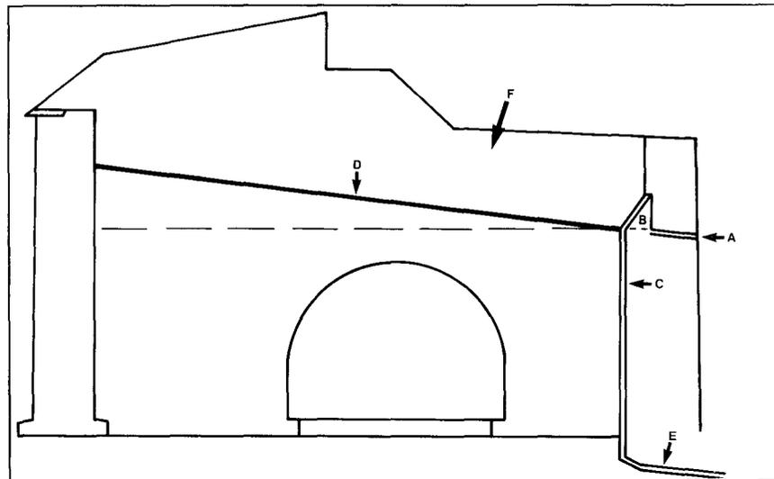
**11** Holloway was using asphalt over the arches, but covered by earth, in conjunction with drains protected from the frost. (a) Old drain blocked up; (b) Masonry to lead water from the rear wall; (c) Drain through pier; (d) Line of gutter on dos d'âne; (e) Underground brick drain; (f) Earth covering. *Redrawn by D. Sullivan.*
