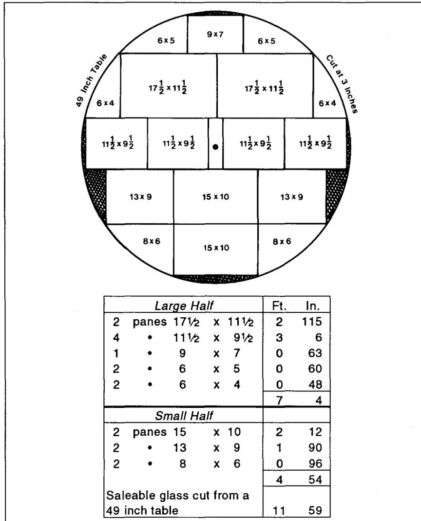
27 Diagram and table showing the panes which might be obtained from a 49-inch table of crown glass. Redrawn by D. Sullivan from illustration in Cooper, *Crown Glass Cutter and Glazier's Manual*, 1835.
