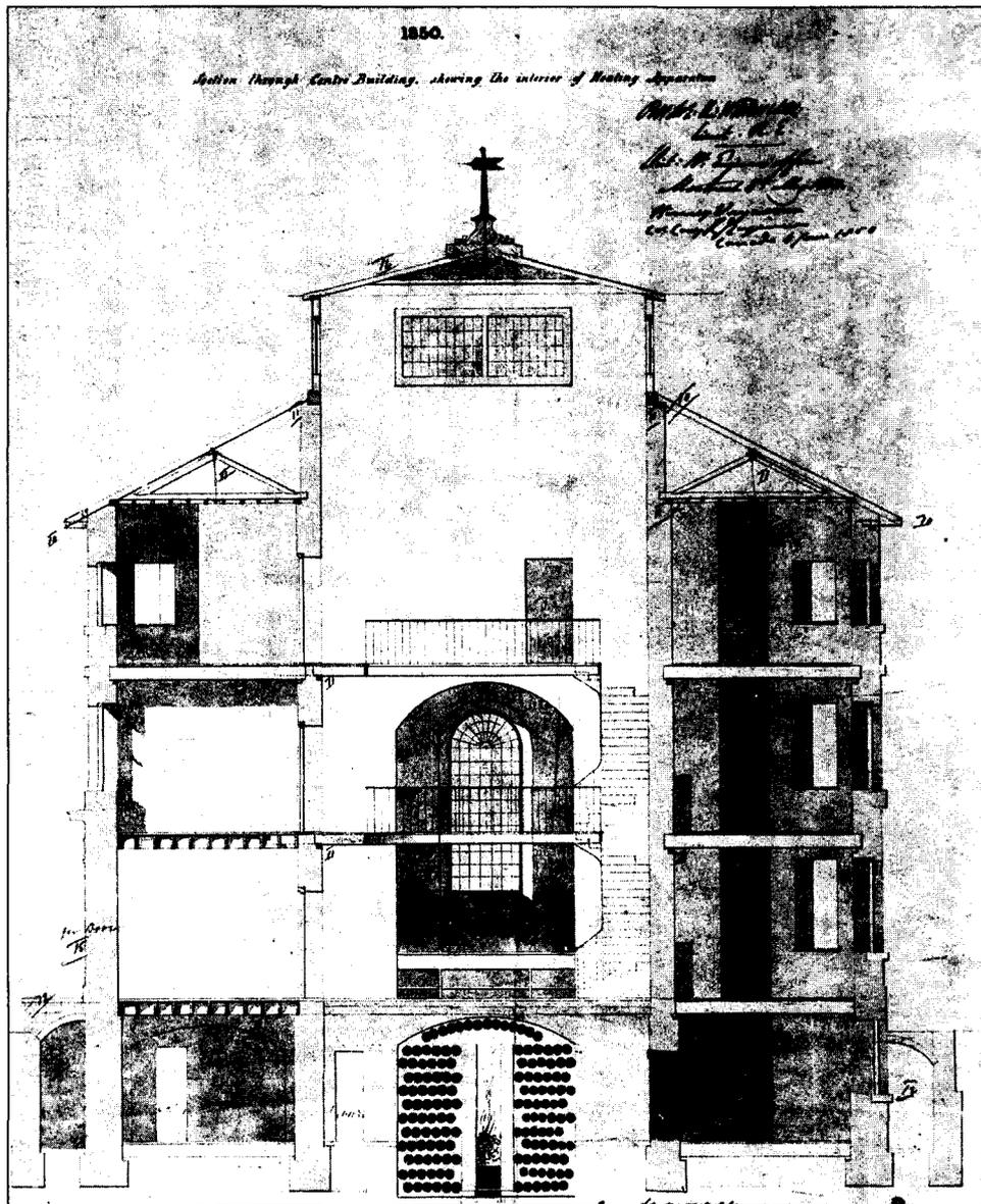
35 Centre Building of the proposed new military prison at Montréal. The long window in the two-storied central corridor is the same as that shown in the printed memorandum on the construction of prisons and barrack cells which was circulated to the various Royal Engineer stations in 1847. The cupola had windows on all sides. The governor's office was in the central portion of the prison. *National Archives of Canada, MG13, WO55/884, f. 201.*
