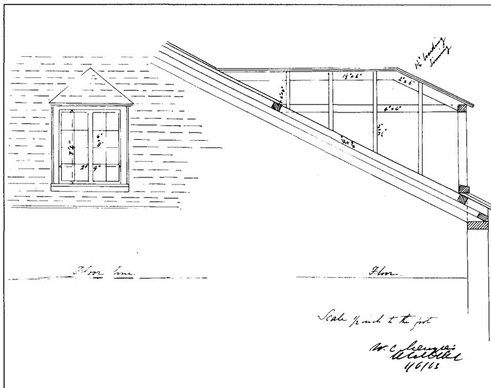
53 Sketch of the type of window proposed for a gunshed at Québec, 1863. The drawing shows how the dormer window was to be constructed. It was to be a casement window, with 8 panes in each half. *National Archives of Canada, RG8, C Series, Vol. 1580, p. 156.*
