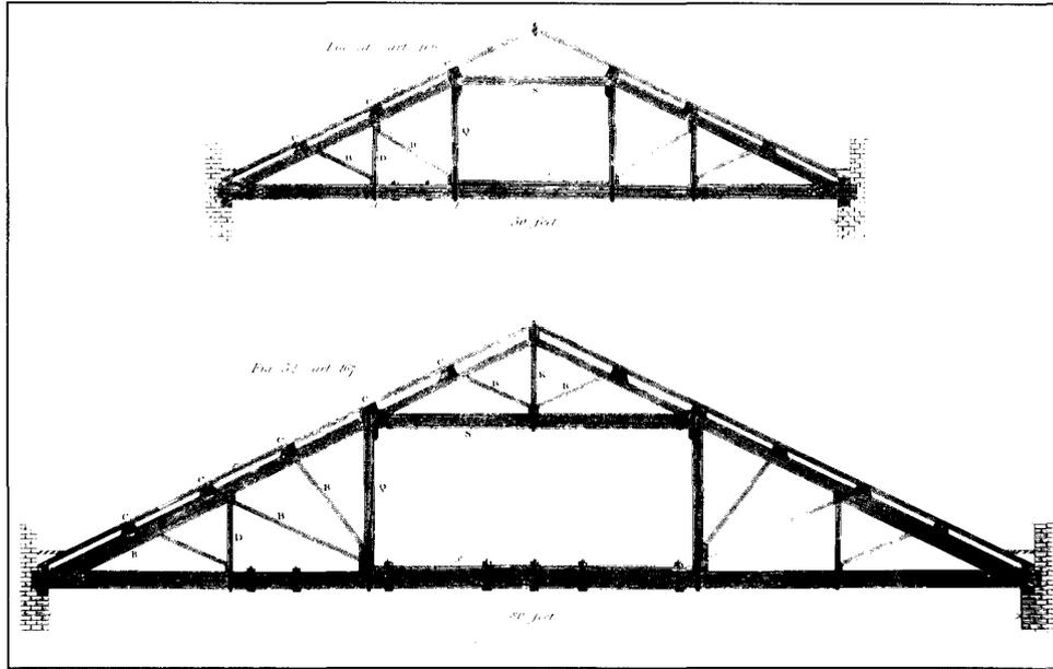
1 Plate from Thomas Tredgold *Elementary Principles of Carpentry* (1853) showing roof construction.
