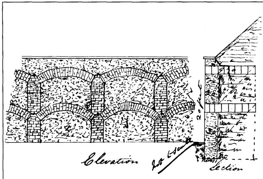
4 This sketch and those in Figures 5, 6 and 7 are from the series of reports written by engineer officers at Halifax describing their work with cement concrete. Here the use of concrete for the front wall of the scarp at Fort Charlotte is shown. In this wall the piers and arches, which were of masonry, were flush with the concrete, but it was suggested that it would have been an improvement to let them project. *National Archives of Canada, RG8, C Series, Vol. 1587, p. 165.*
