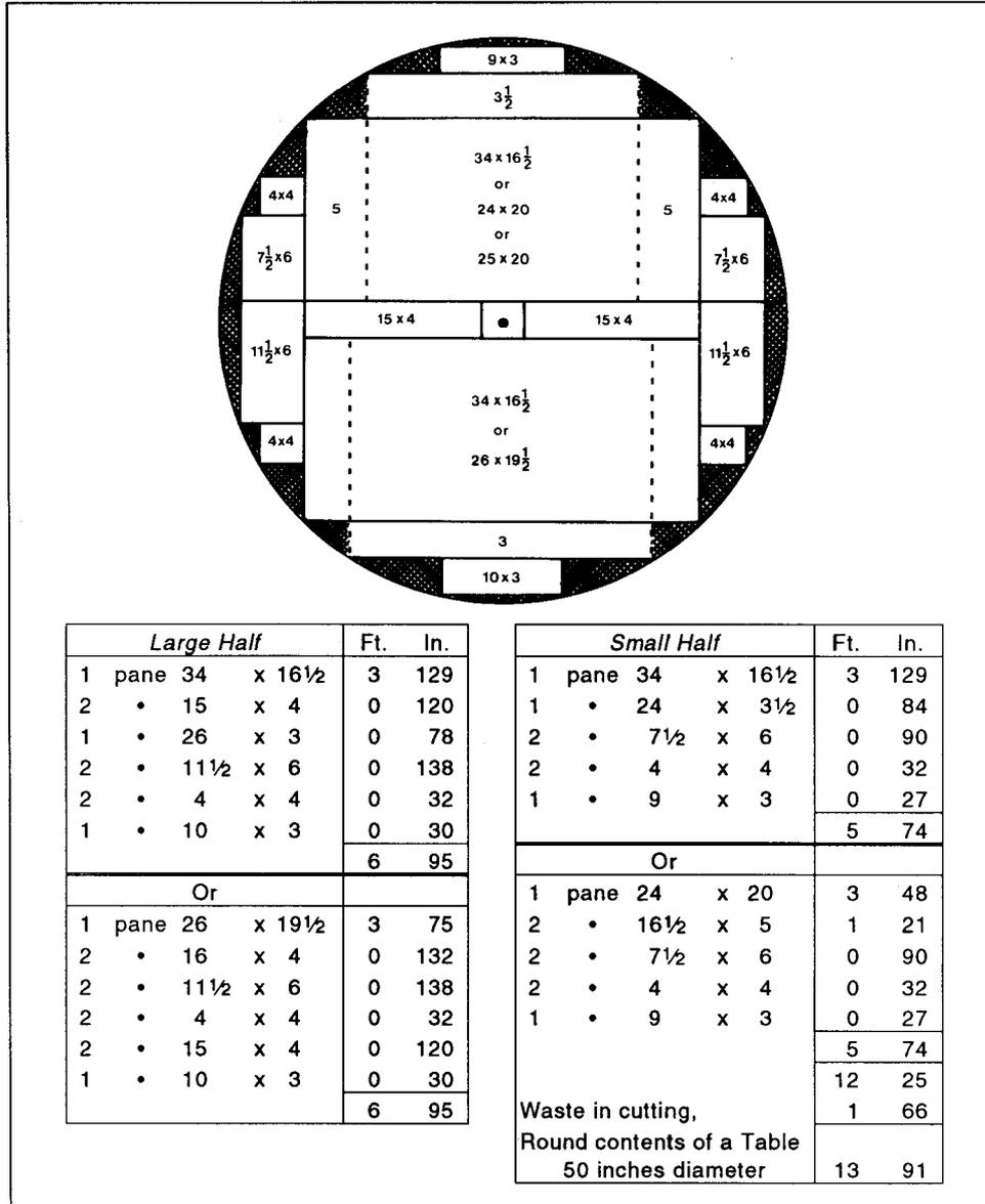
28 Diagram and table showing the panes which might be obtained from a 50-inch table of crown glass. Redrawn by D. Sullivan from an illustration in Cooper, *Crown Glass Cutter and Glazier's Manual*, 1835.
