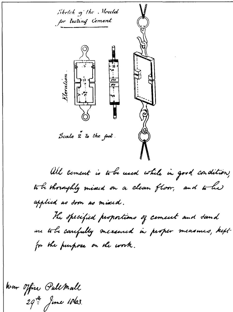
2 Sketch of the mould to be used for testing cement by the Royal Engineers, 1863. National Archives of Canada, RG8, C Series, Vol. 1649, p. 252.
