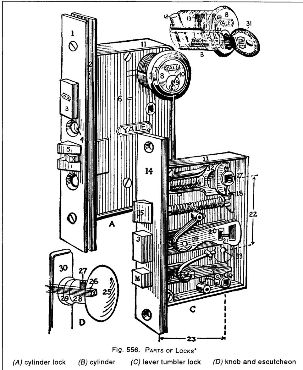
17 Modern mortice locks. The lever tumbler lock is a three-bolt lock. The gating can be seen (21) through which the projection on the bolt can pass when the tumbler is raised the correct amount. *Voss and Henry, Architectural Construction.*
