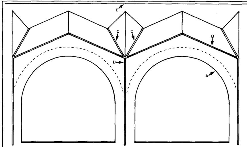
**10** This and Figure 11 are taken from Holloway's letter to the Inspector General of Fortifications, May 1844. (a) Casemate arch; (b) Dos d'âne, asphalted; (c) Gutters; (d) Drain pipe through pier of arch; (e) Parapet. *Redrawn by D. Sullivan.*
