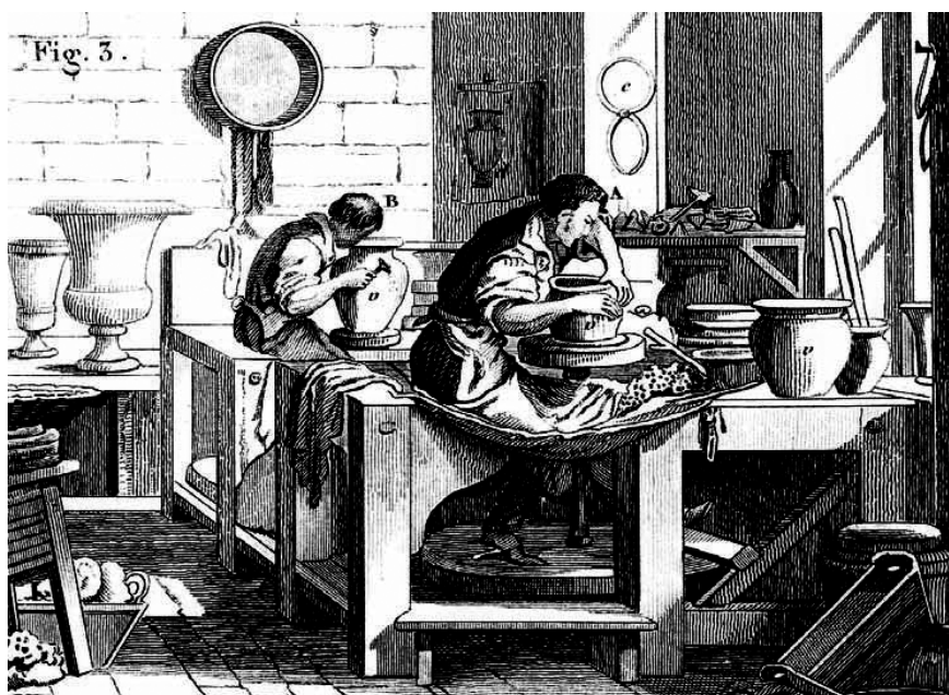
Figure 7. Wheel throwing. The worker in front is shaping and his colleague behind is turning, (i.e., finishing) the object (Brongniart 1844:plate 45).
