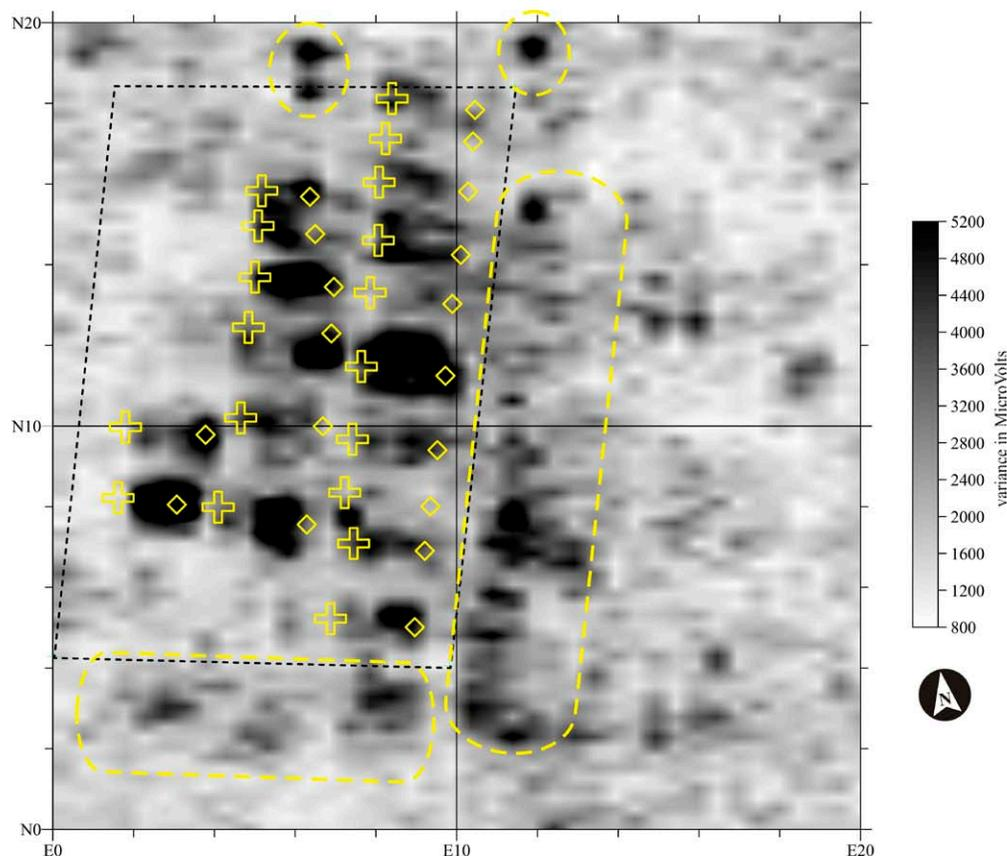
**Figure 2.** Time slice (plan view) map of GPR survey results from the Ellis Cemetery. The Ellis Cemetery dates from the mid-19<sup>th</sup> century. It is on what is now Fort Bragg, North Carolina. Graves in this family cemetery are not as closely spaced as those in most public cemeteries, and individual graves are generally well defined. Less distinct patterning outside the modern fence suggests the possibility of unmarked burials (Jones and Maki 2003).
