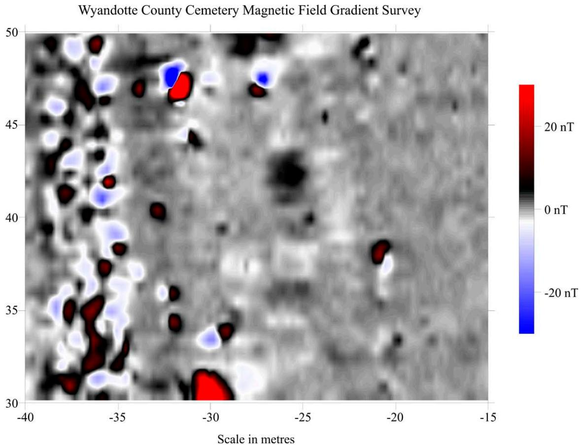
**Figure 6.** Wyandotte County Cemetery magnetic survey (detail). This data plot illustrates a variety of different magnetic expressions of graves (reflecting different burial practices) and other cemetery patterning. Specific interpretations are given in Figure 7. These data are part of a larger multi-method investigation as discussed in the case study.
