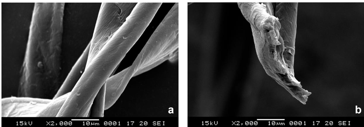
**Figure 4.** SEM images showing: (a) the longitudinal morphology of Jinta fibers under 2000× magnification; (b) the cross-sectional morphology of Jinta fibers under 2000× magnification. (Photos by authors, 2006).
