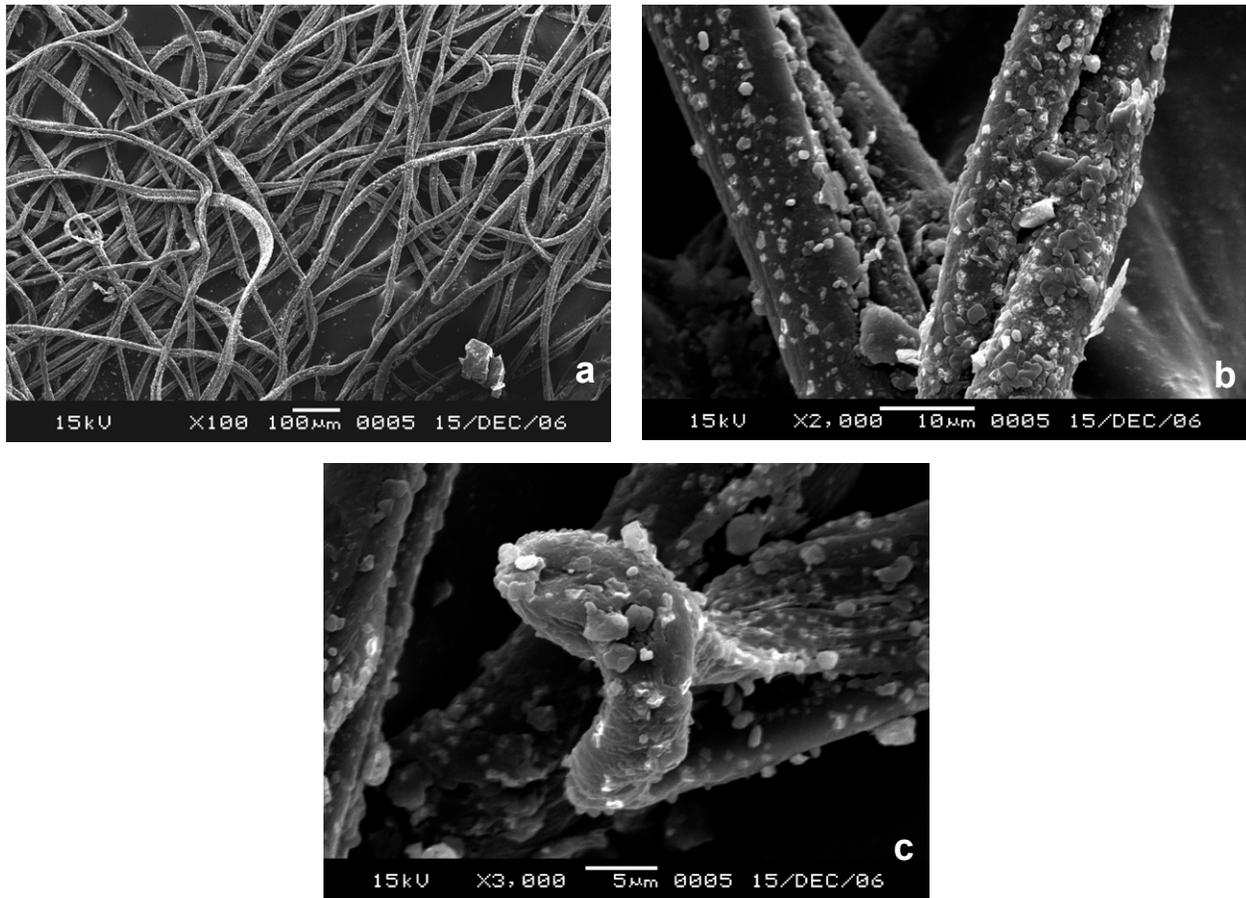
**Figure 3.** SEM images showing: (a) the longitudinal morphology of the unearthed fibers under 100× magnification; (b) the longitudinal morphology of the unearthed fibers under 2000× magnification; (c) the cross-sectional morphology of the unearthed fibers under 3000× magnification. (Photos by authors, 2006).
