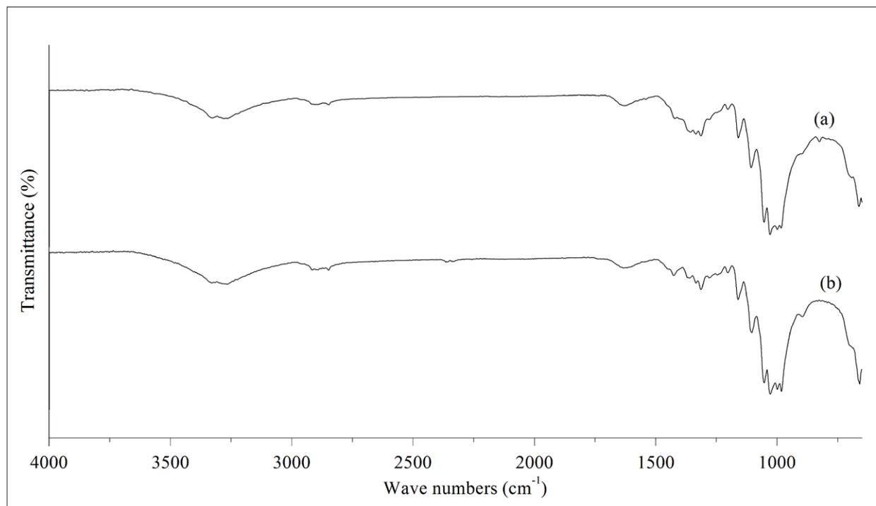
**Figure 5.** IR spectra of samples: (a) Unearthed, (b) Jinta. (Drawing by authors, 2007).
