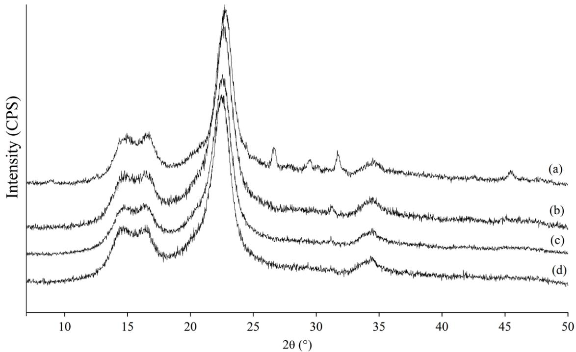
**Figure 6.** XRD spectra of samples: (a) Unearthed, (b) Jinta, (c) SXY-1, (d) TM-1. (Drawing by authors, 2007).
