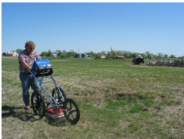
Ground-penetrating radar survey of the Nicodemus School site.
