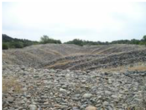
FIGURE 2. Typical bucket-line dredge tailings.
