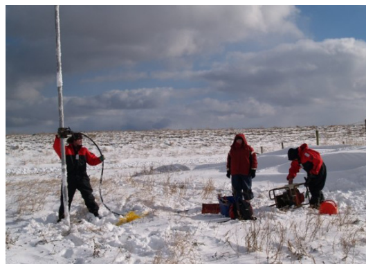
Katie Cottreau-Robins and David Scott work with graduate student Peter van Hengstum to drive a vibracore into the dikeland soils. A modern outer dike stands in the background.
