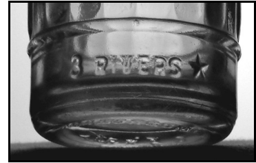
Figure 6-11 – 3 RIVERS {star} manufacturer’s mark on heel
