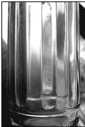
Figure 6-13 – Vent marks on embossed specialty bottle
