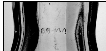
Figure 7-24 – Code sequence on skirt; the first two digits (55) are the date code
