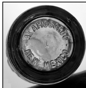
Figure 7-25 – Baseplate of the 1955 bottle made by the Laurens Glass Works; note the dot spacers
