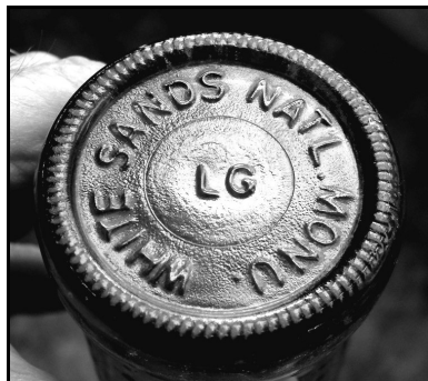
Figure 7-37 – Base of Sprite bottle with the White Sands designation and the L-G mark
