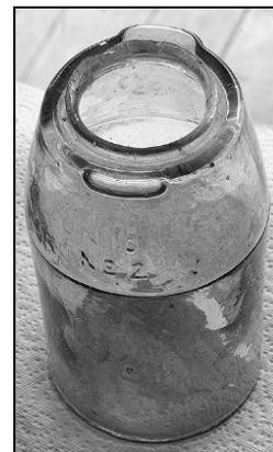
Figure 24 – Finish of Union jar; note mold seams (Courtesy of North American Glass)
