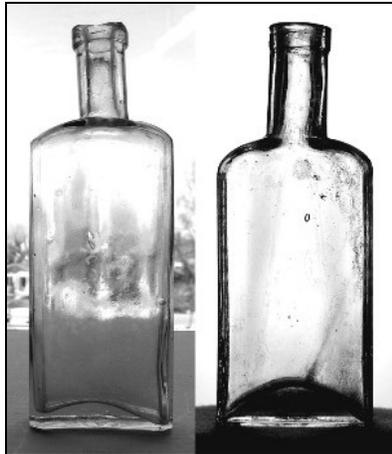
Figure 22 – Comparison of Type I Circle-A bottle (left) and Type II A.G.W. bottle (right)
