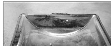
Figure 17 – Fin at the intersection of the base and heel
