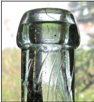
Figure 1 – Groove with squared bottom (eBay)
