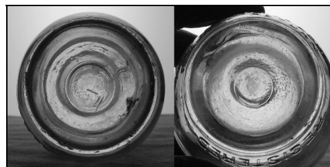
Figure 9 – Basal scars – C.H.B.CO (left); Mass C (right)
