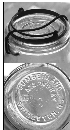
Figure 15 – Safety jar base & finish (North American Glass)
