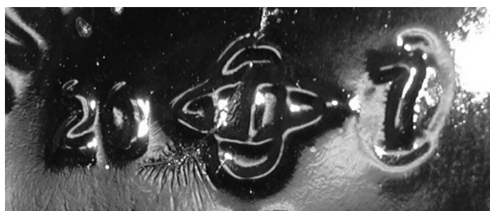
Figure 2-2 – Peened and re-stamped date code on Owens-Illinois base (Tucson Urban Renewal Collection)
