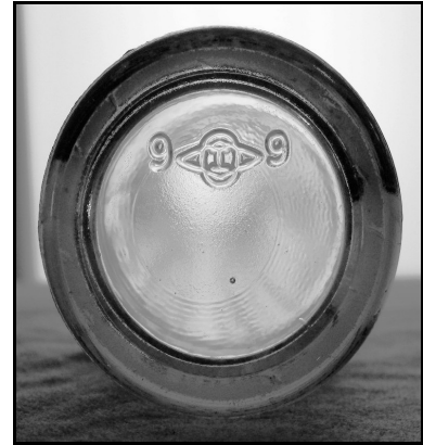
Figure 5-91 – Base with Owens-Illinois label and codes
