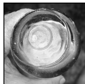
Figure 7-23 – Base of the unusual bottle, showing atypical machine scars
