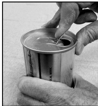
Figure A-24 – Depressing the tear-strip
