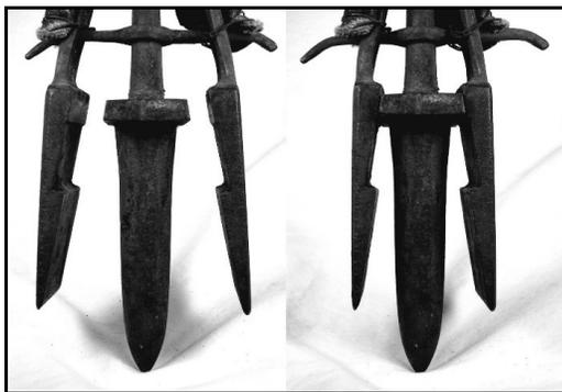
Figure 2-36 – Finishing tool used to make one-part finishes in open and closed positions (Lindsey 2012)
