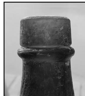
Figure 2-31 – Two-part finish with rounded lower ring
