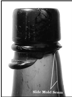
Figure 2-51 – Extreme example of slop-over in an applied finish
