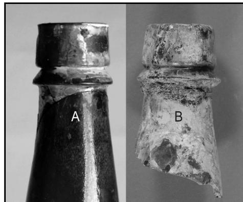
Figure 2-30 – Two-part finishes with sharp lower rings: A – flared; B – wedge
