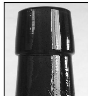
Figure 2-37 – Finish made by a tool similar to the one in Figure 36 (Lindsey 2012)
