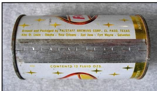
Figure 8b-9 – Seam of 13-notch can
