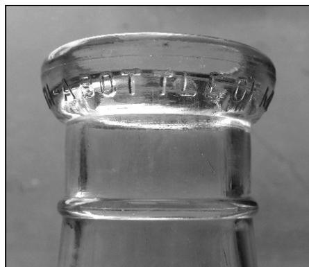
Figure 10-26 – Finish roll of Escobar embossed bottle
