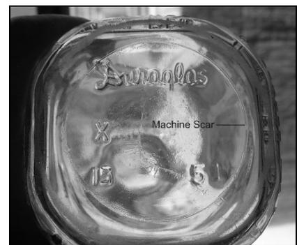
Figure 2-38 – Base showing later machine scar
