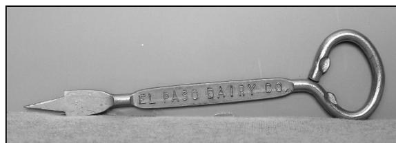
Figure 4-22 – Combination cap pick and bottle opener
