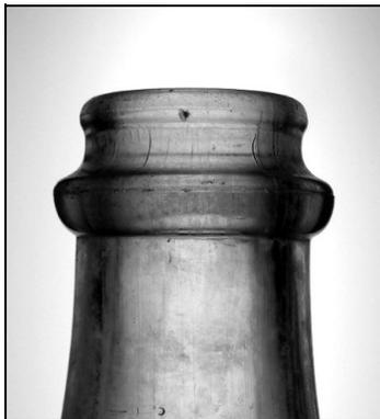
Figure 5-26 – Later Dacro finish with bumper roll
