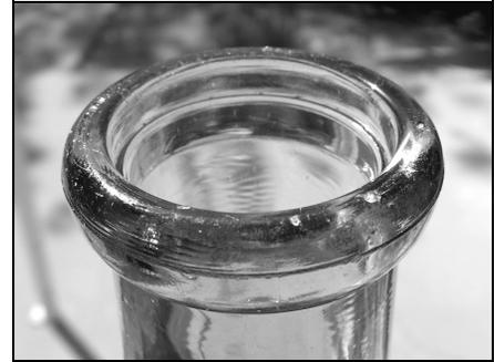
Figure 5-6 – Early Common Sense (cap-seat) finish
