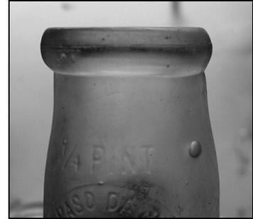
Figure 6-21 – Offset finish on machine bottle
