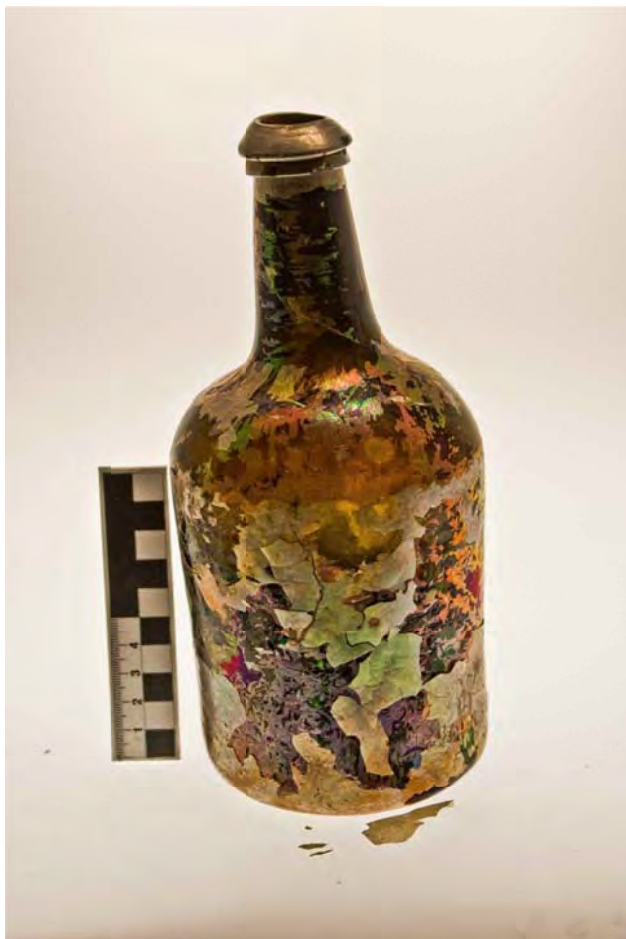
Figure 49. Example of devitrification on St. George artifact. Note scaling.
