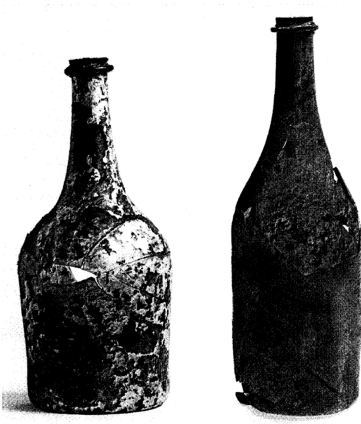
Figure 73. After Jones and Smith, 1985. Jones and Smith identify both artifacts as “French wine” bottles. They date bottle at left as “...[m]id-18th century;” bottle at right as “early 19 th century.” Bottle on right, at 281mm height and base diameter of 91mm, directly corresponds to the St. George champagne family both metrically and visually. Image not to scale.
