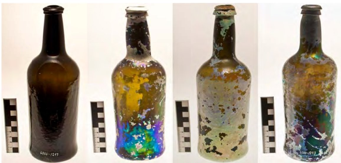
Figure 50. One pristine artifact (far left) compared with three others in various stages of devitrification.
