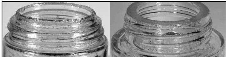
Figure 40 – Finish comparison; insert-and-band (left); glass screw cap (right) (North American Glass)
