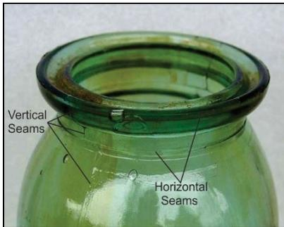
Figure 55 – Offset finish seam (North American Glass)
