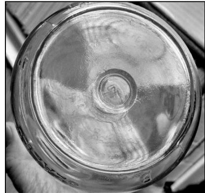
Figure 5 – Ejection scar date code (eBay)
