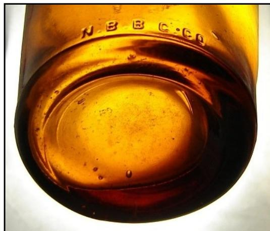
Figure 3 – Machine heelmark (eBay)
