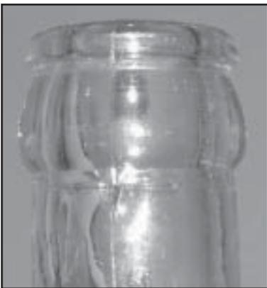
Figure 2: Root Semiautomatic Bottle Finish
