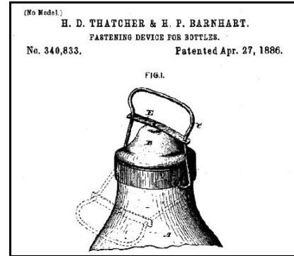
Figure 3 – Thatcher and Barnhart’s patented lid (Patent #340,833)
