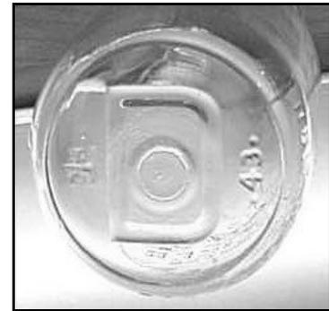
Figure 21 – 1943 date code with MTC Mark on Base (eBay)
