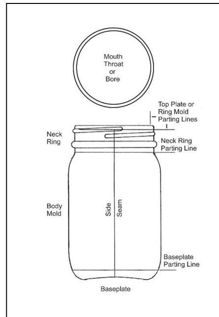
Figure 15 – Types of parting lines and seams on a jar
