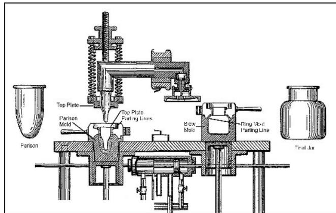
Figure 26 – Detail of molds from the Ripley’s first jar machine patent, plus parison and finished jar
