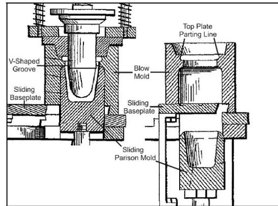
Figure 28 – Detail of molds from one of Blue’s early patents (No. 567,071)
