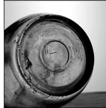
Figure 21 – Ejection or valve scar
