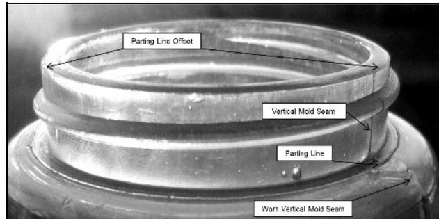
Figure 42 – Characteristics – including V-shaped groove – on early Mason jars
