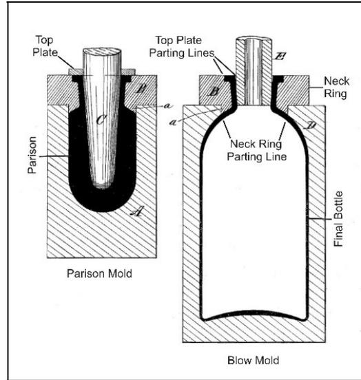
Figure 25 – Detail of molds from the Arbogast patent
