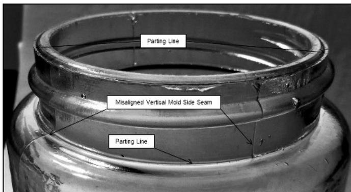
Figure 43 – Characteristics on -ATLAS- / MASON'S / PATENT jar
