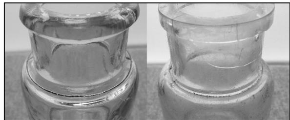
Figure 35 – V-shaped grooves just below neck/shoulder joint
