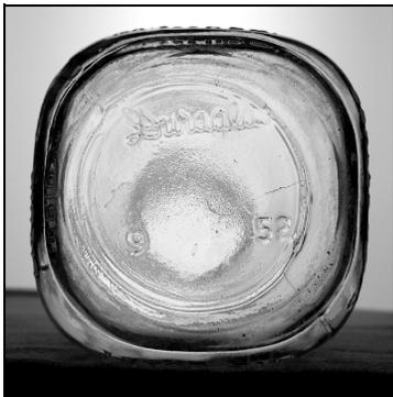
Figure 22 – Typical blow-and-blow machine scar
