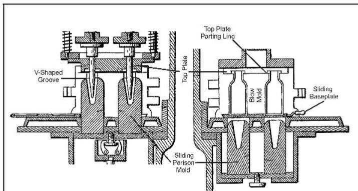
Figure 31 – Detail of one of Blue's double-mold patents (No. 682,906)
