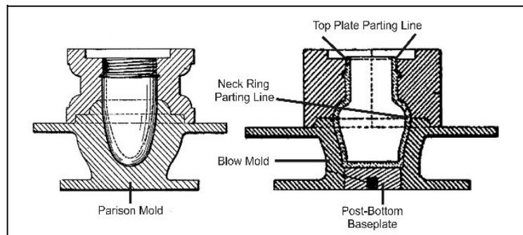
Figure 27 – Detail of molds from the Ripley's second jar machine patent
