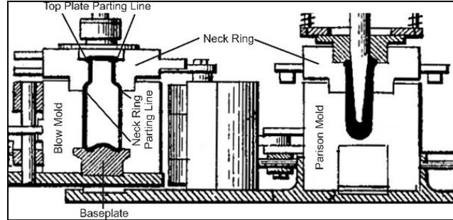
Figure 29 – Detail of molds from one of Blue’s second set of patents (No. 917,947)
