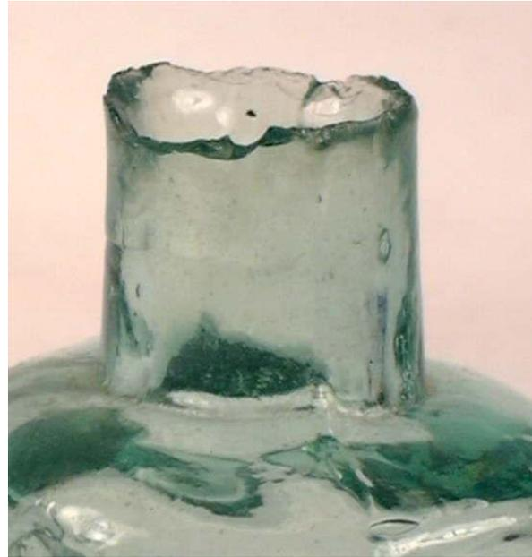
*(Figure 3 [to right]. A raw, non-manipulated, burst-off finish on an early 20<sup>th</sup> century English ink bottle. This looks very similar to the raw, cracked-off finish (Fig. 2) but does have some subtly differing characteristics.*
