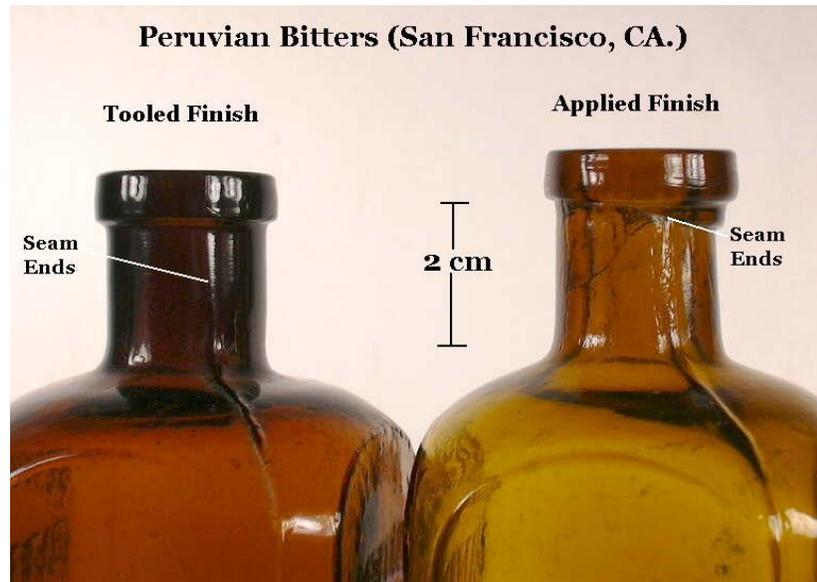
the mold, the finish shape and bore conformation was made more precise—to ensure proper closure fit—with minor re-firing and/or tooling of the extreme upper portion of the finish (Deiss 1981).
