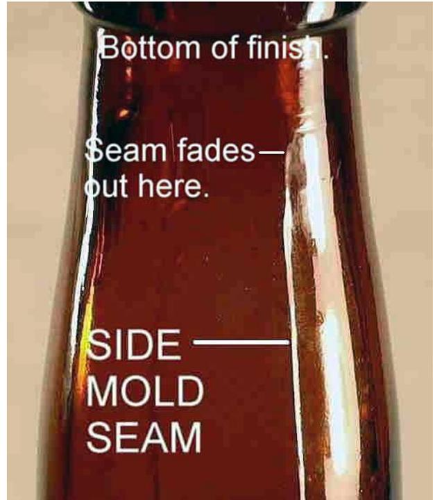
(Figure 20 [to right]. Neck of a bottle, showing horizontal striations eliminating the upper end of the vertical side seam below the finish, a characteristic indication of a tooled finish.)
