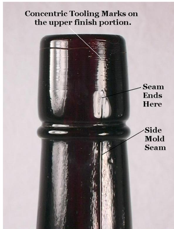
(Figure 23 [to left]. An improved tooled finish on an early 20th century liquor bottle. The lower part of the finish is formed in the mold, and only the upper portion is tooled.)
