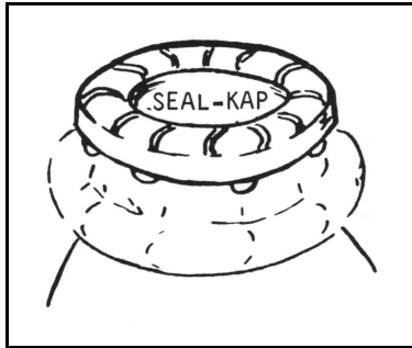
Figure 3-29 – Seal-Kap closure (Rawlinson 1970:33)
