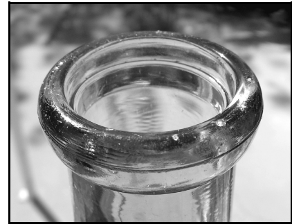
Figure 3-2 – Early Common Sense (cap-seat) finish
