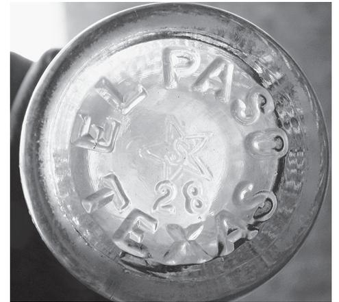
**Figure 8: Star-S with a two-digit date code**
