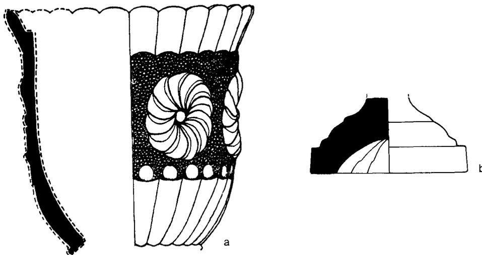
**Figure 14.** (a) A press-moulded bowl showing the characteristic features of press moulding. (b) "Lemon-squeezer" foot which would have been manufactured in a hand-held presser and attached to a stemmed vessel. The "plunger" was decorated with the lemon-squeezer design which is on the underside of the foot.
