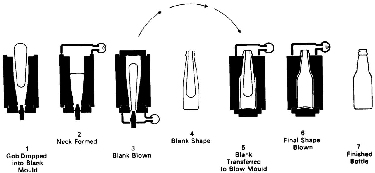
**Figure 17.** Mechanical forming of glass containers: the blow-and-blow process. (Published with permission of Glass Manufacturers Federation 1973: 25.)
