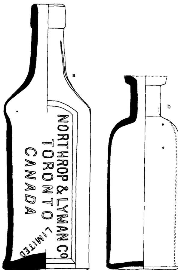
**Figure 29.** Two bottles blown in vented moulds. (a) Has one vent mark on the shoulder and the bumpy appearance of the letters is accounted for by vent holes in many of the letters. (b) Has two vent marks on the shoulder with two more on the opposite side of the bottle.
