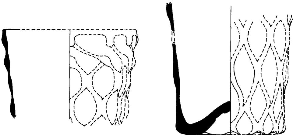
**Figure 12.** This tumbler has been manufactured by pattern moulding. The diamonds are more concentrated at the bottom of the object and diffused at the top, and the interior and exterior glass surfaces have corresponding contours (cf. contact-moulded examples, Fig. 5).
