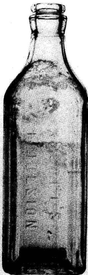
**Figure 148.** Kork-n-seal finish. The bottle illustrated has a finish designed to take a kork-n-seal lever-type cap.
