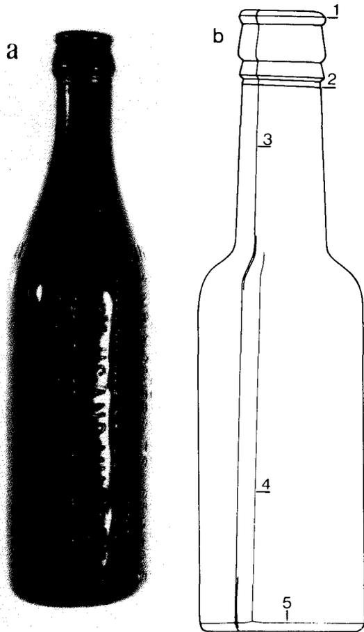
Figure 19. Two bottles showing typical machine-produced mould seams, including, on (b), a "ghost" seam from the parison mould on the body.
