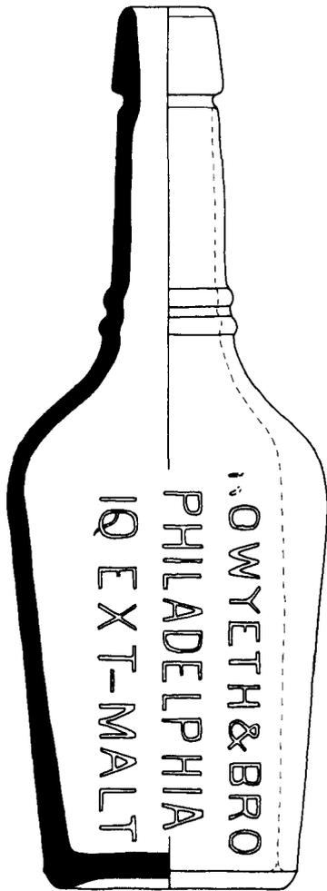
**Figure 9.** A probable bitters bottle blown in a two-piece mould with a separate base part that leaves a mould seam above the heel of the bottle.
