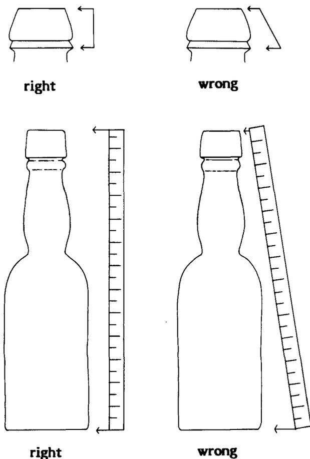
Figure 83. Taking measurements.
