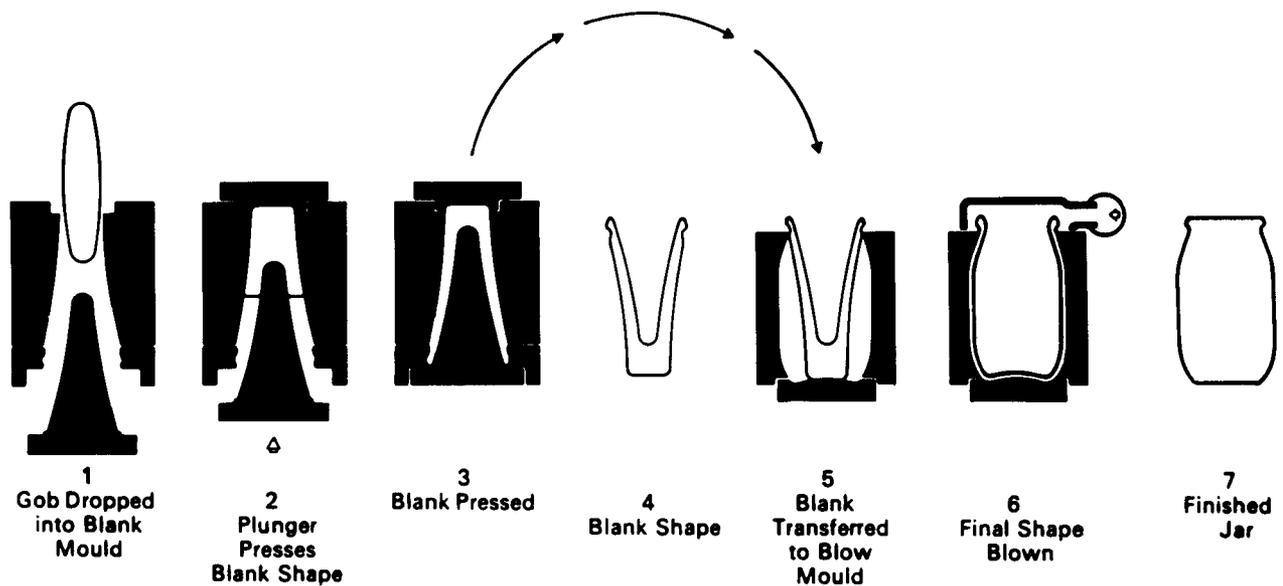
**Figure 18.** Mechanical forming of glass containers: the press-and-blow process. (Published with permission of Glass Manufacturers Federation 1973: 25.)
