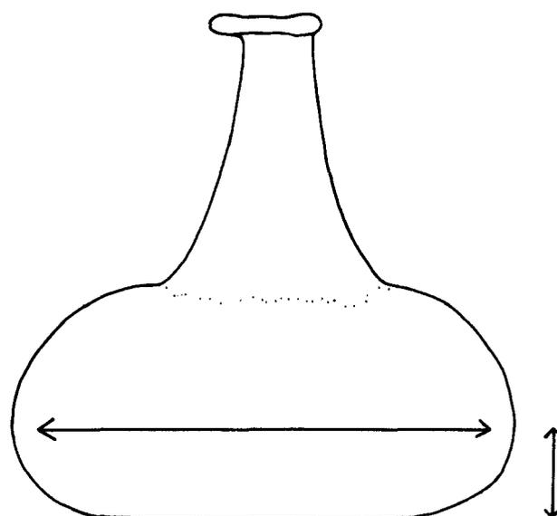
Figure 96. Maximum body dimension and height of maximum body dimension.
