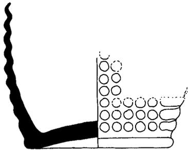
**Figure 5.** Examples of contact-moulded glassware. Note that the interior and exterior surfaces of the glass are parallel to each other.
