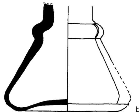
**Figure 27.** (a) The base of this bottle has been formed by an oval-shaped post and the body shaped in a two-piece mould. (b) An ink bottle manufactured by a two-piece mould and separate cup base mould.
