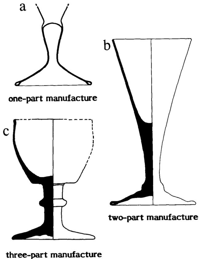
**Figure 100.** Stemware manufacture. (a) One-part manufacture. The entire object is formed from one gather of glass. (b) Two-part manufacture. The bowl and stem are formed from one gather of glass, the folded foot from another. (c) Three-part manufacture. Bowl, stem, and foot are formed from separate gathers of glass.
