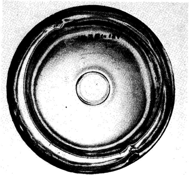
**Figure 23.** A valve mark on a bottle base. Toulouse (1969: 583) says that this mark is caused by a valve that ejects the parison out of the mould so that it can be transferred to the blow mould for completion.
