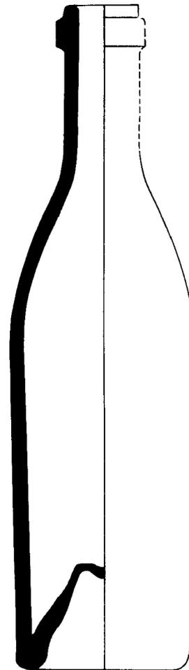
**Figure 11.** A probable champagne bottle manufactured by turn moulding. Note the symmetry throughout the bottle parts.
