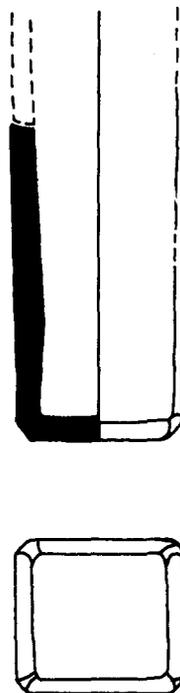
**Figure 31.** Square perfume bottle with chamfered corners, the body and base formed by cutting.
