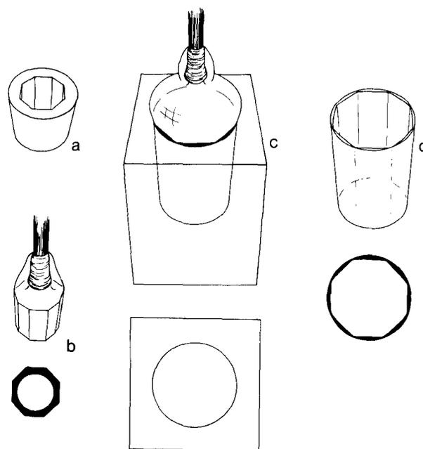
**Figure 13.** The process of optic moulding, based on Larsen, Riismøller, and Schlüter (1963: 389). (a) The part-sized mould with a pattern of panels. (b) The pattern-moulded parison. (c) The parison expanded in a smooth unpatterned dip mould. (d) Finished tumbler with the panel pattern on the inside of the object and a smooth exterior.
