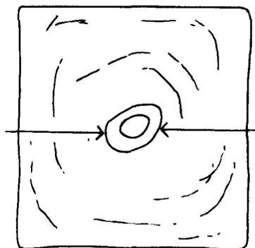
Figure 99. Pontil mark diameter.
