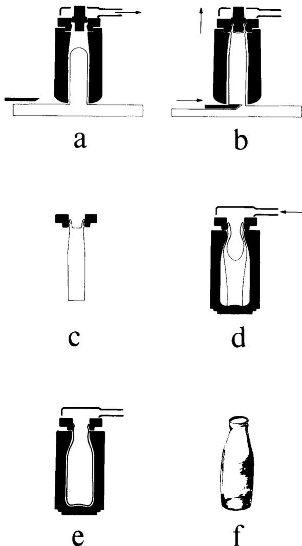
**Figure 16.** Mechanical forming of glass containers: the Owens suction-and-blow process. (a) The gob is sucked up into the blank mould. (b) The neck of the container is formed and the glass gob sheared off at the base. (c) The blank or parison shape with the ring mould still attached. (d) The blank shape is transferred to a full-sized mould and blowing begins. (e) The container's final shape is blown. (f) A finished bottle.
