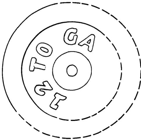
**Figure 26.** A separate base part which has left its own mould seam on the heel of the bottle. Separate base parts do not always have commercial markings.
