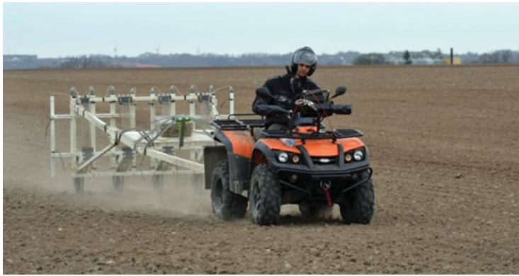
FIGURE 1. Motorized magnetometer survey with an array of 10 sensors spaced at 25 cm intervals. This system was towed at approximately 15–20 km/hr over the fields. In the background the crest of the ridge, on which the square structures were detected, can be seen. (Photo by Immo Trinks.)
